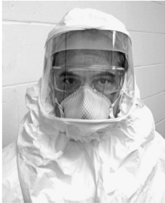
Fig 1. N95FFR and protective eyewear used in tandem with a loose-fitting (shrouded) powered air-purifying respirator. (Photograph courtesy of the National Institute for Occupational Safety and Health/National Personal Protective Technology Laboratory/NIOSH.)
